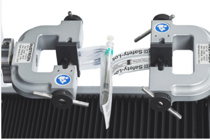
Figure 2. Image of Universal Testing Machine grips from Instron®. https://www.instron.com
